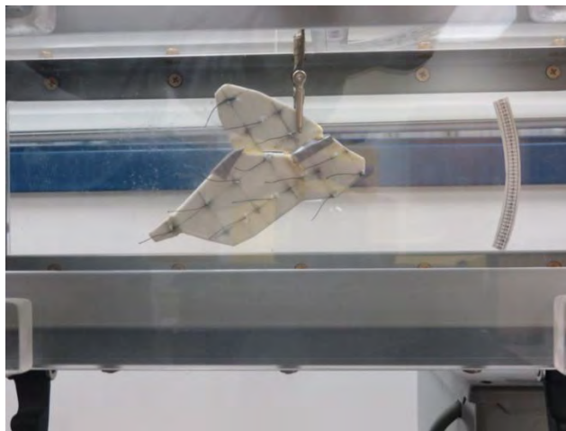
The model of Tapejara wellnhoferi being tested in the wind tunnel.
